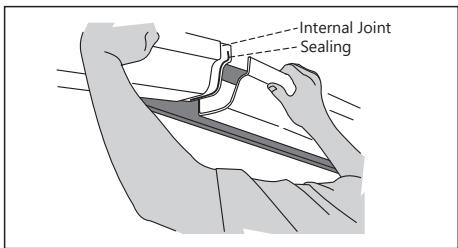
Make sure each sealing lace is in contact with each one of the pieces which are being united (gutter or miter).
