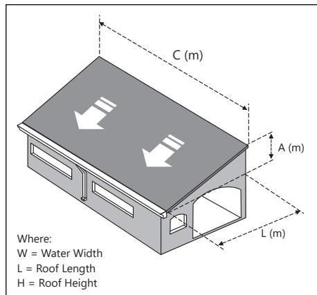
For roofs with inclination of 20°, the maximum area by nozzle (RMA) which gutter can exhaust on the main regions is given by the Pluviuometric Intensity (PI) calculation.
