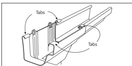
Note that this attachment allows for gutter movement inside outlet nozzle. This freedom of movement is necessary to absorb gutter dilation and contraction, which naturally occurs with ambient temperature variation.
