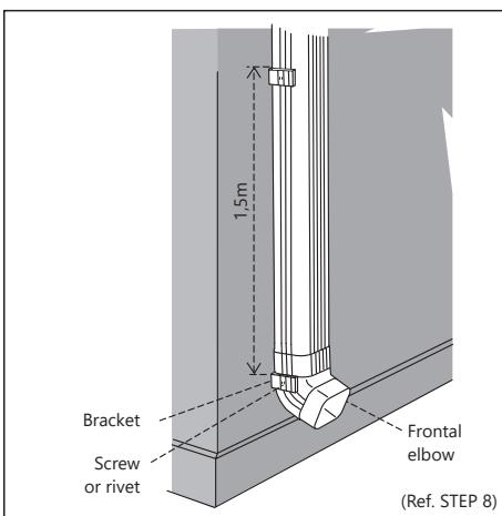
Begin assembly by letting last support loose so it is possible to connect the last support. If necessary, keep this last extremity suspended using a string.
